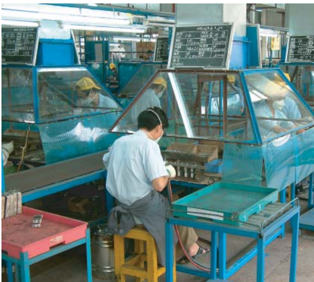
Soldering the battery plates
